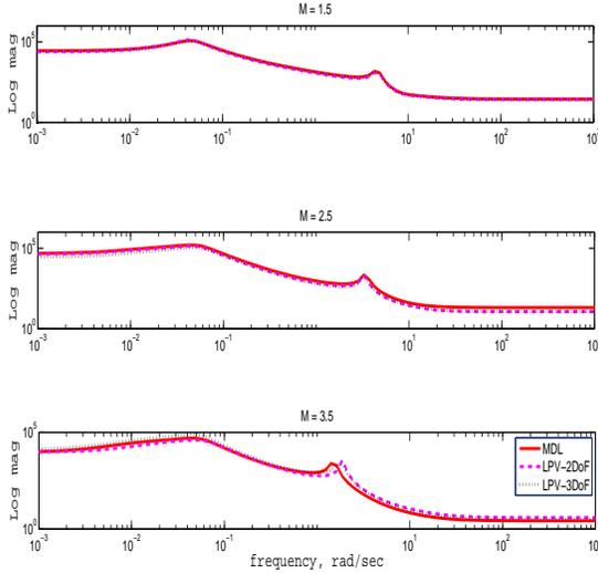
Fig. 7. LTI, LPV-2DoF fit & LPV-3DoF fit: frequency responses
