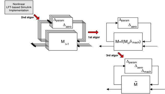
Fig. 6. LPV/LFT modeling tool process
