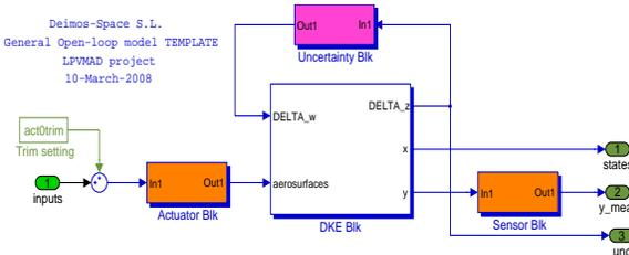
Fig. 3. Open-loop nonlinear main-layer Simulink template shell
