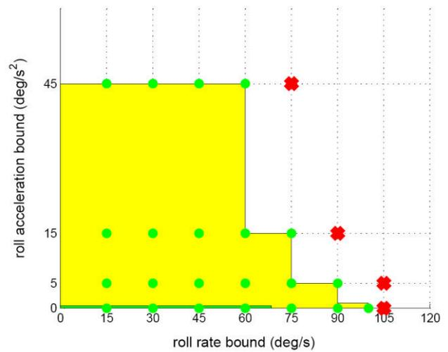
Fig. 6. IQC robust stability region (yellow) vs.  $\mu$  analysis results (green line @ zero roll acceleration).
