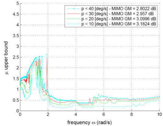
Fig. 4. Multi loop GM and associated roll rate levels.
