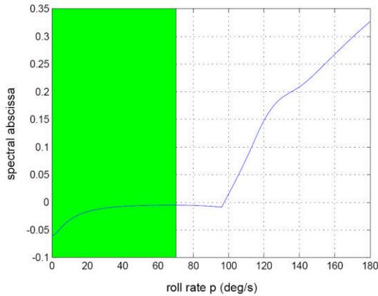
Fig. 2. Stability degree vs. positive roll rate (blue line). Mu results are given by the shadowed region (in green).
