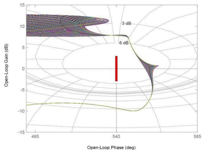
Fig. 5. Nichols chart corresponding to roll rates  $|p| \leq 15$  degrees per second. The red area represents the minimum GM guaranteed by mu analysis.
