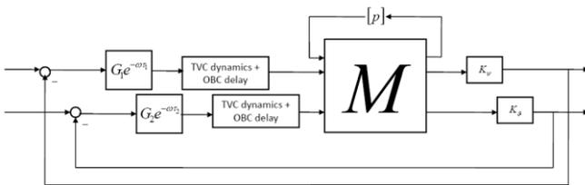
Fig. 3. MIMO closed-loop LFT with TVC dynamics, OBC delays, and artificial gains  $G_*$  and time delays  $\tau_*$ .
