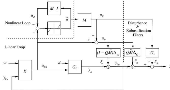
Fig. 5. Analytical representation of the robust AW architecture.
