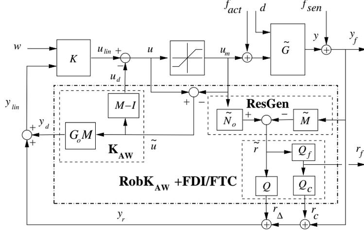
Fig. 7. General Robust AW architecture with FDI/FTC capability.
