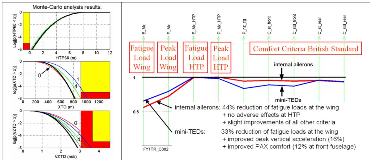
**Fig. 3** Visualization of Monte-Carlo criteria optimization for automatic landing controller (left) [24] and of optimization criteria for gust load alleviation and comfort improvement design (right) [25].
