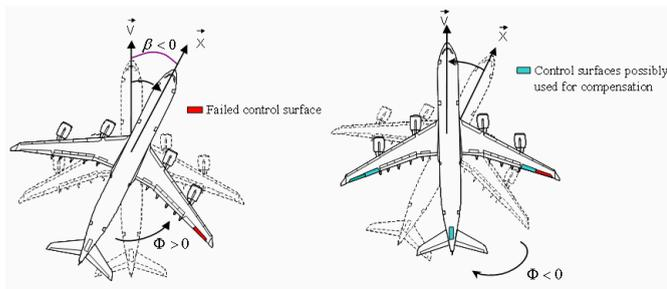
Figure 2 Effect of aileron jamming and potential control surfaces used for compensation
