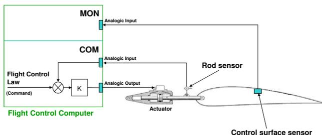
Figure 1 Actuator and sensor localization in the control loop
