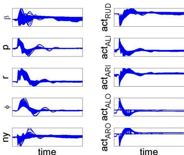
Figure 9 System and control responses: Yaw-Angle, ARI, S1.1
