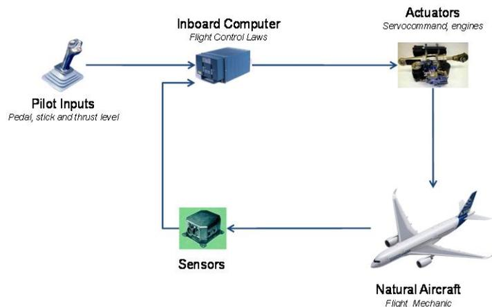
Figure 2 Closed-loop aircraft model main components<sup>4</sup>
