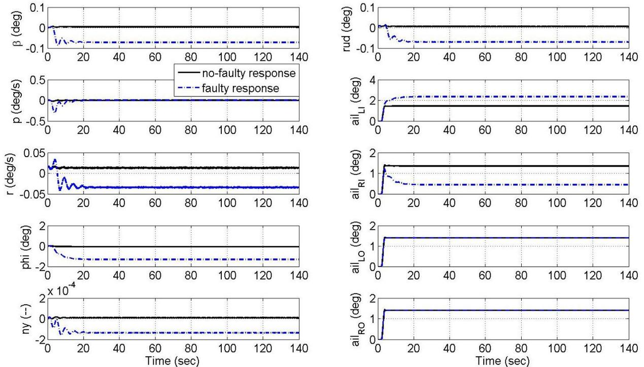
Figure 8 Nonlinear time domain simulation (ADDSAFE-FES): FDI inputs
