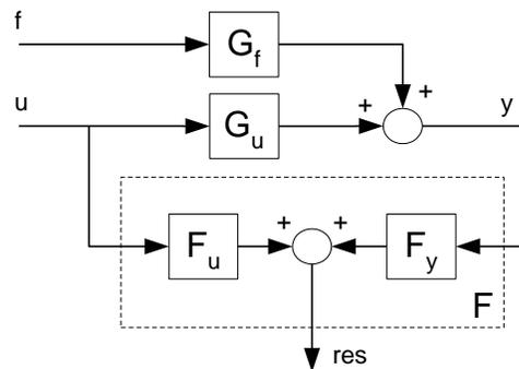
Figure 5 Basic model-based FDD design architecture
