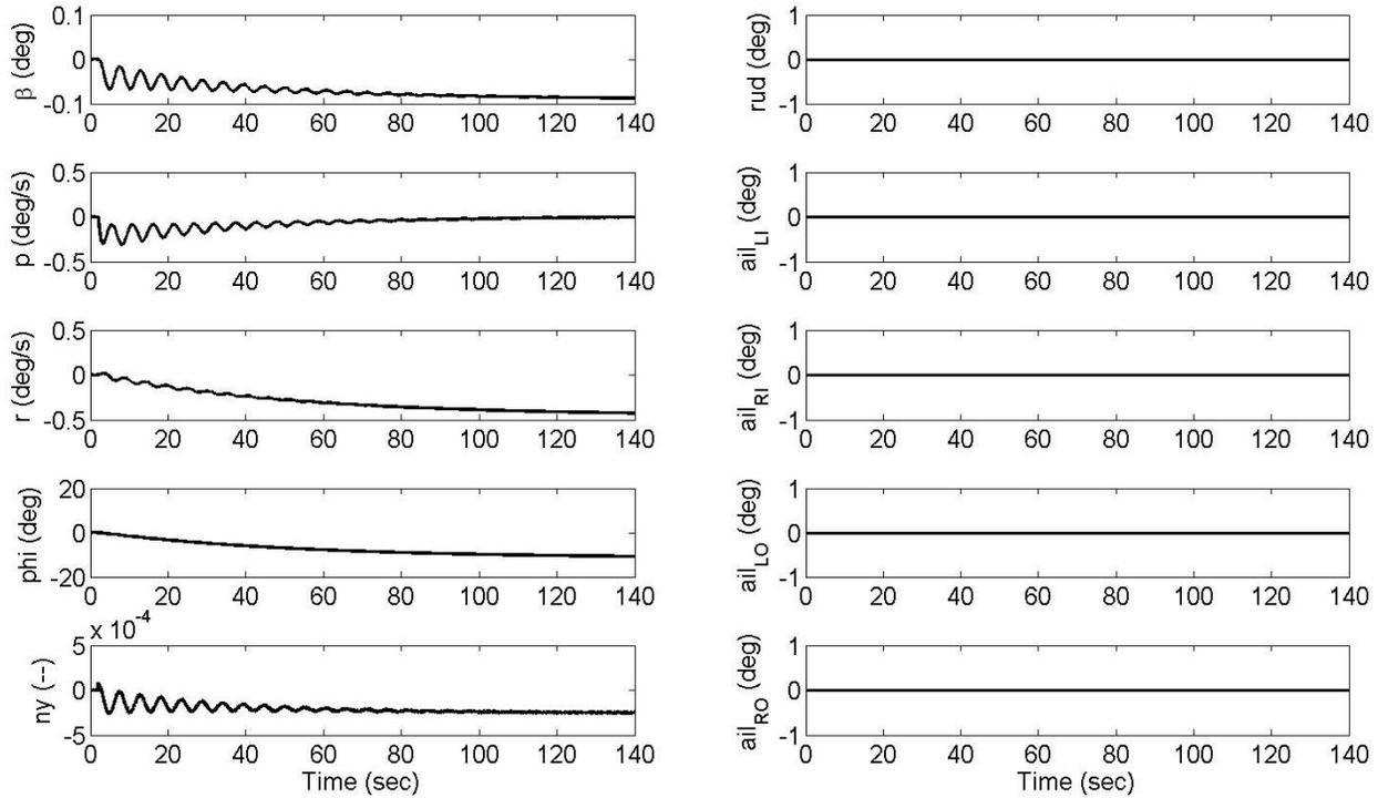
**Figure 6 Linear (with full nonlinear actuator model and faults) time domain simulation: FDI inputs**
