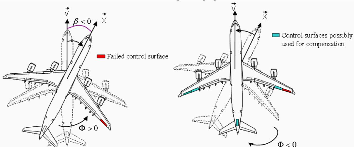
**Figure 3 Effect of the aileron jamming and control surfaces possibly used to compensate<sup>4</sup>**
