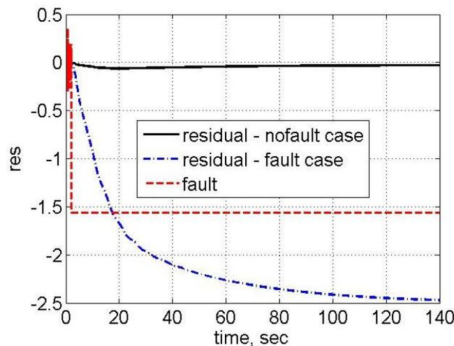
Figure 9 Nonlinear time domain simulation (ADDSAFE-FES): FDI residual & fault
