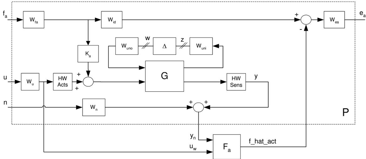
**Figure 13. Longitudinal H-infinity FDI filter design interconnection.**
