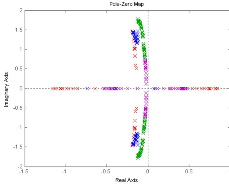
**Figure 8. Migration of the longitudinal short period mode poles for the nominal trimmed vehicle (red – [0,20]s; blue – [20,50]s; green – [50,100]s; magenta – [100,130]s)**
