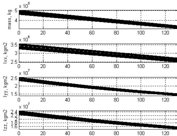
Figure 5. Ascent period (0-130 sec) mass and inertia for 50 random ascent simulations.
