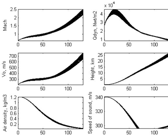
**Figure 3. Ascent period (0-130 sec) environmental parameters for 50 random ascent simulations.**
