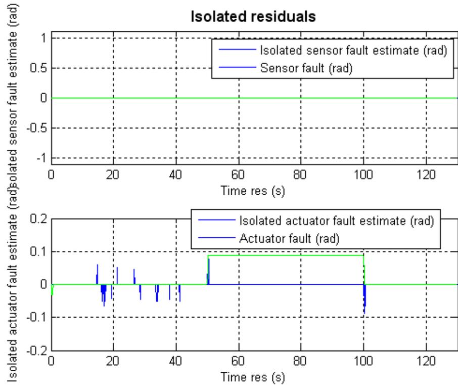
Figure 17. Isolated fault estimates for 1000 run MC campaign for the engine 2 pitch gimbal bias fault.
