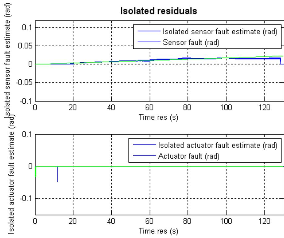
Figure 16. Isolated fault estimates for 1000 run MC campaign for the yaw rate sensor drift fault.
