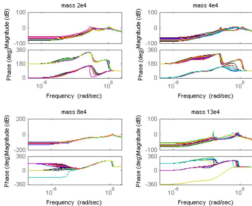
**Figure 7. Effect of parameter uncertainty on the effective outer elevator to pitch rate ( $q$ ) frequency response at four trim points in ascent flight at four flight conditions: 25 random plant cases.**
