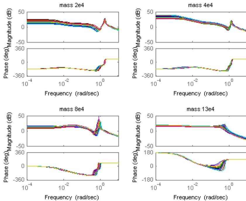
**Figure 9. Effect of parameter uncertainty on the effective outer aileron to roll rate (p) frequency response at four trim points in ascent flight at four flight conditions: 25 random plant cases.**
