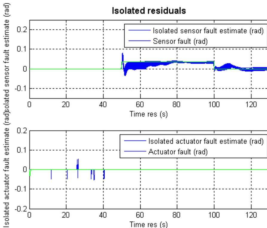
**Figure 15. Isolated fault estimates for 1000 run MC campaign for the yaw rate sensor bias fault.**
