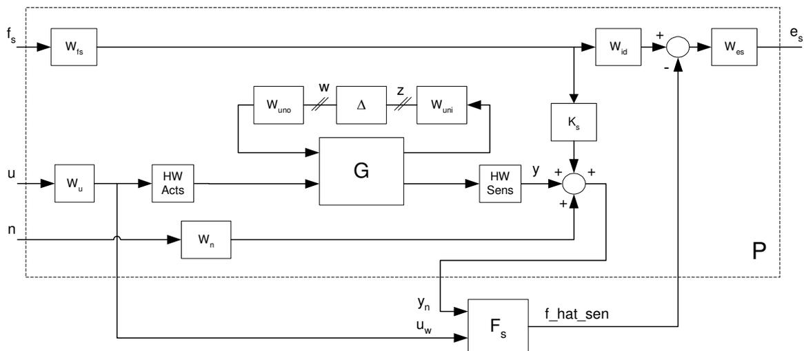
**Figure 14. Lateral H-infinity FDI filter design interconnection.**
