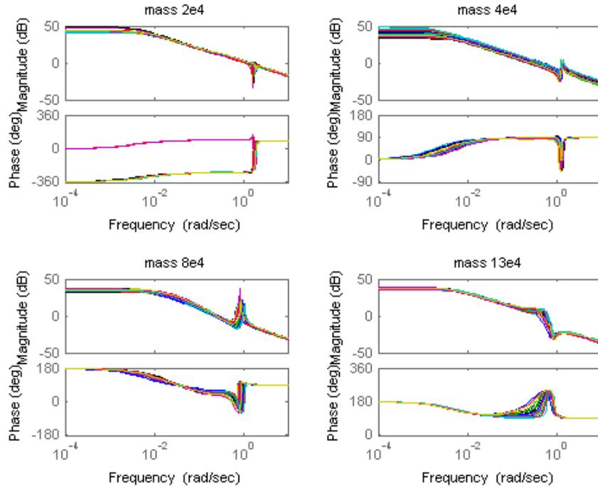
**Figure 10. Effect of parameter uncertainty on the rudder to yaw rate ( $r$ ) frequency response at four trim points in ascent flight at four flight conditions: 25 random plant cases.**
