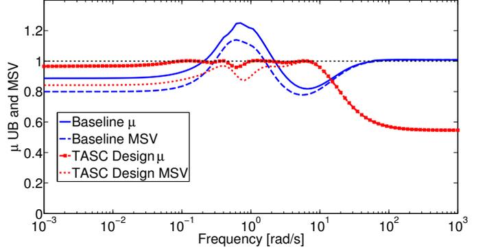
Fig. 5. Lateral Plant RP with two different controllers
