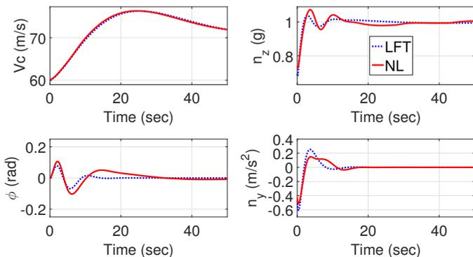
Fig. 2. Nonlinear time-domain validation of the full LFT
