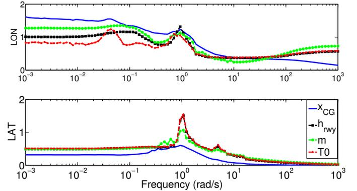
Fig. 9. Sensitivity of RP to the uncertain parameters for Longitudinal and Lateral plant
