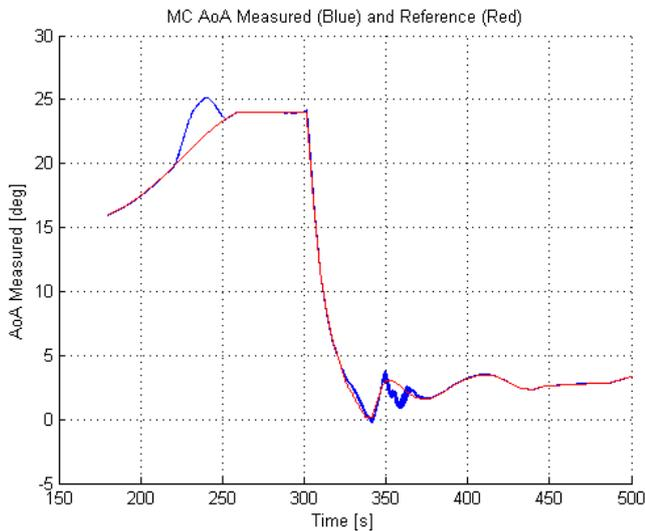
Fig. 6 Angle of attack measured without compensation vs Angle of attack reference.
