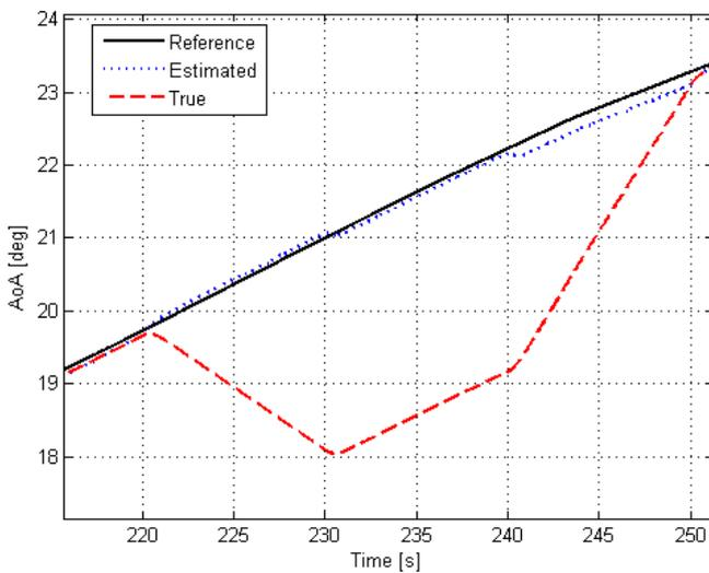
Fig. 3 Evolution of the Angle of Attack in the fault scenario without any compensation
