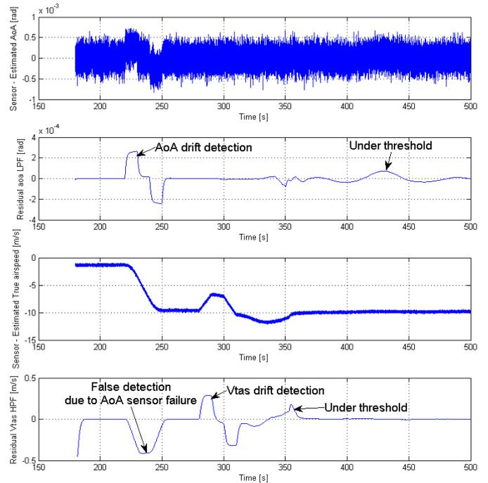
Fig. 4 Raw residual Angle of Attack and Vtas signals before and after a low pass filter and high pass filter respectively
