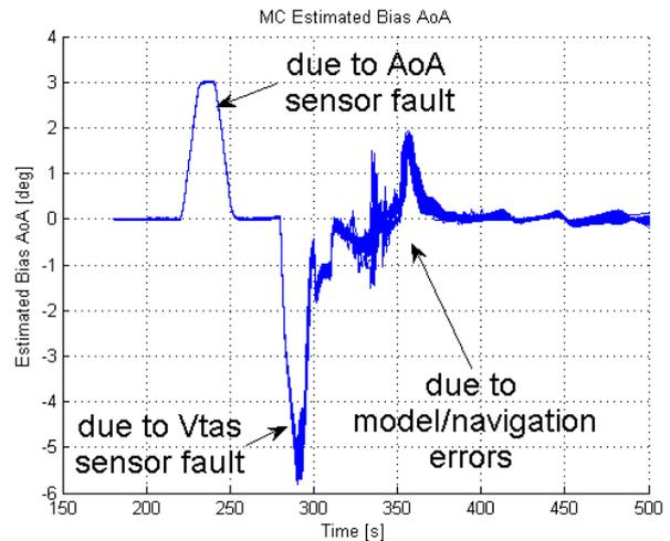
Fig. 8 Estimation of the bias of the Angle of Attack.
