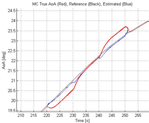
Fig. 9 True (Red), Estimated (Blue) and Reference (Black) Angle of Attack during the failure period.
