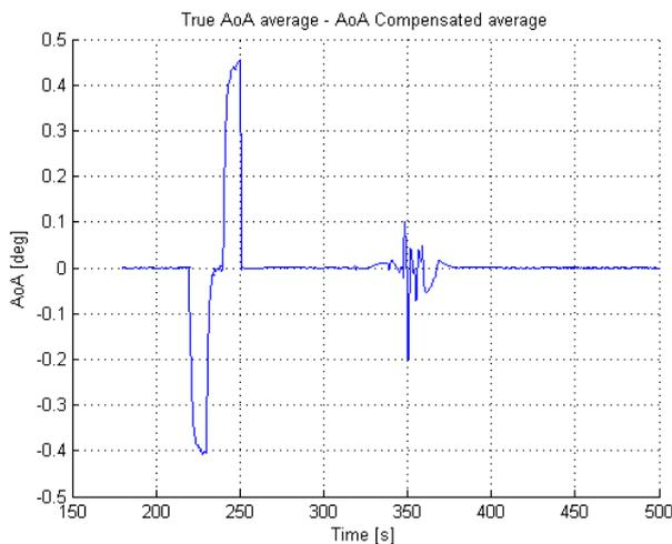
Fig. 10 Error between True and Compensated averages of Angle of Attacks.
