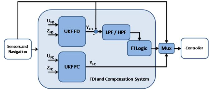
Fig. 2 FDIR System architecture, where LPF and HPF are Low and High pass filters respectively.
