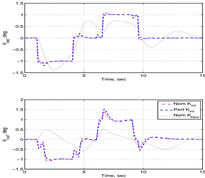
Fig. 7. Actuator signals for integrated and non-integrated designs
