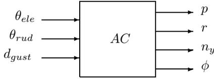
Fig. 2. Aircraft block diagram
