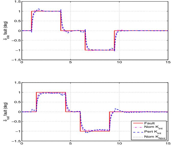
Fig. 5. Fault detection for integrated and non-integrated designs
