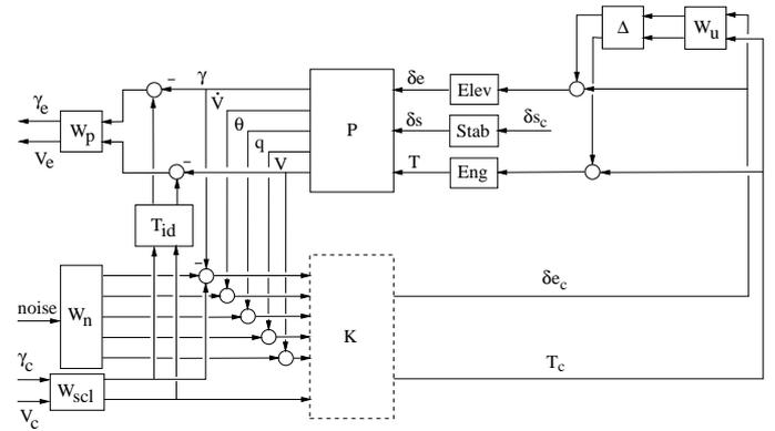
Figure 2: Interconnection structure for  $K_{NF}$  and  $K_F$ .
