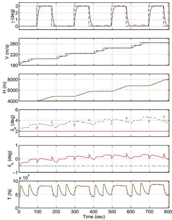
Figure 4: Aircraft responses for LPV controller during normal operation ( $K_{NF}$  - dashed) and with full elevator fault ( $K_F$  - solid). Commands are in dashdot lines.
