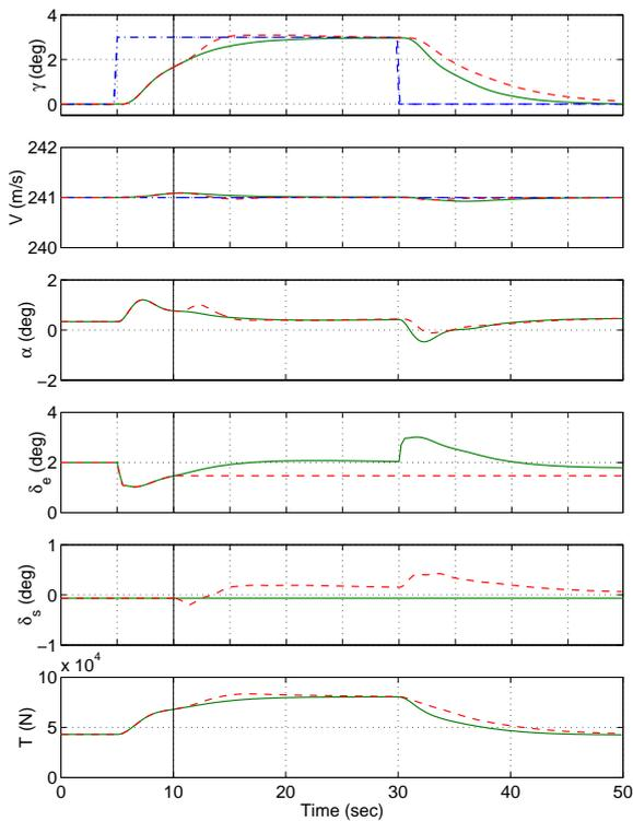
Figure 5: Aircraft responses for  $K_R$  with elevator-lock at 10 sec. (Commands: dashdot; normal: solid; locked: dashed).
