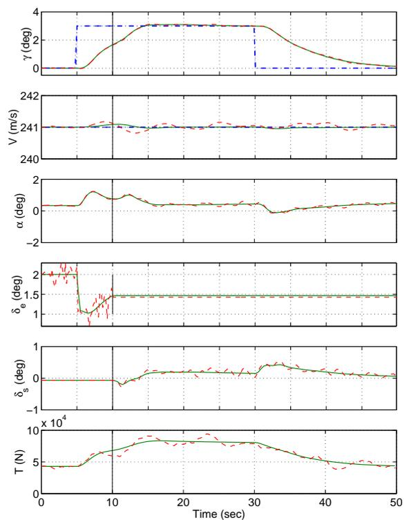
Figure 7: Aircraft responses for  $K_R$  with elevator-lock at 10 sec with sensor noise and wind gust. (Commands: dashdot; locked: solid; with disturbance: dashed).
