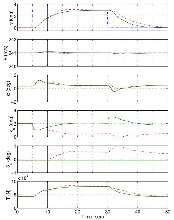
Figure 6: Aircraft responses for  $K_R$  with elevator-float at 10 sec. (Commands: dashdot; normal: solid; float: dashed).
