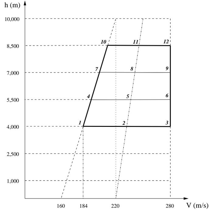
Figure 1: B-747 Up-and-Away flight envelope — trapezoidal area enclosed by bold lines.
