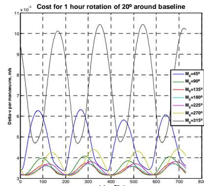
Figure 2-4 Centralised rotation of  $20^\circ$  around baseline, cone aperture angle of  $4^\circ$ .  $\Delta V$  for a manoeuvre duration of 1 hour
