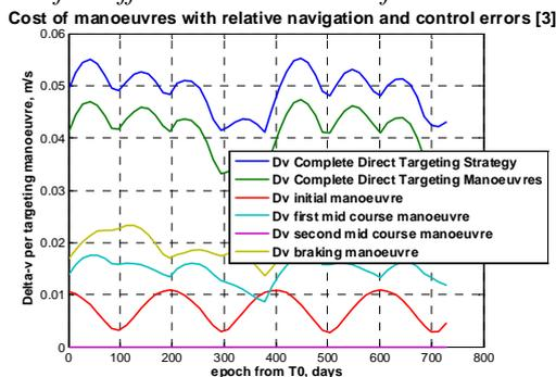
Figure 2-7 DV during the complete mission timeline for a DT with 1 MCM @ 0.5 h before the target and using Optical Metrology for the first manoeuvre.
