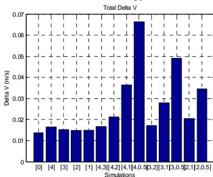
Figure 2-6 Comparison of DV of DT manoeuvres (top) for different combinations of MCMs
