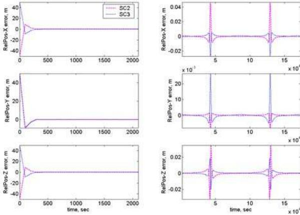
Figure 3-5 Closed Loop baseline: relative position error w.r.t. SC1 in LVLH frame
