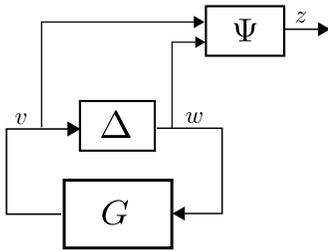
Fig. 1. Augmented plant for ROA analysis.
