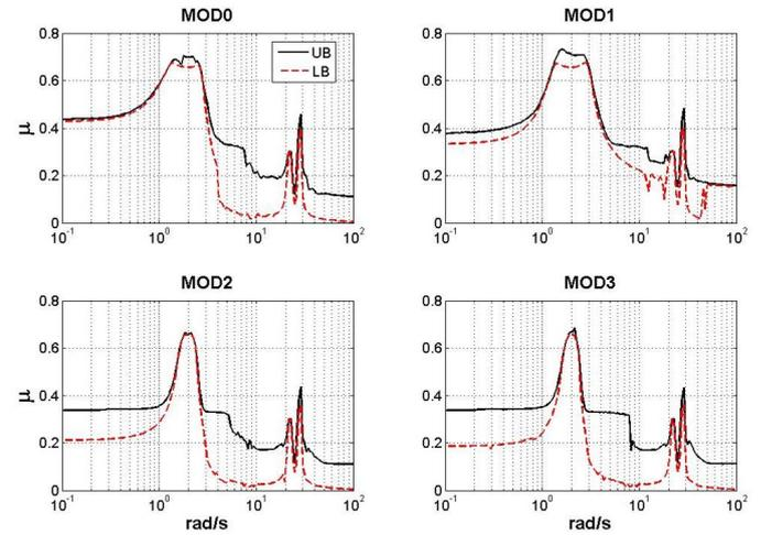
Fig. 4.  $\mu_{RS}$  bounds for all LFT models with no bending  $\Delta$
