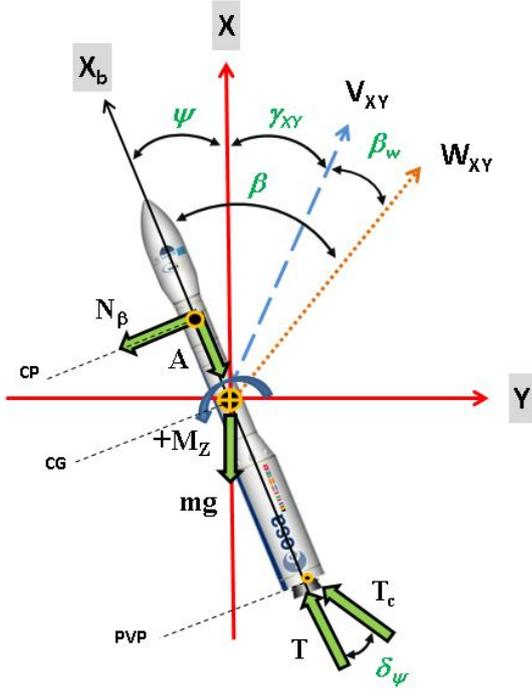
Fig. 4. VEGA yaw-motion diagram
