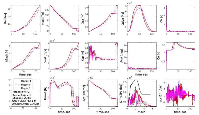
Fig. 6. VGCTRL time responses for  $\delta_{T_c}=[-1, 0, 1]$  and  $k=[-1]$
