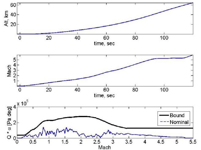
Fig. 3. VEGA mission profile: altitude, Mach and  $Q\alpha$
