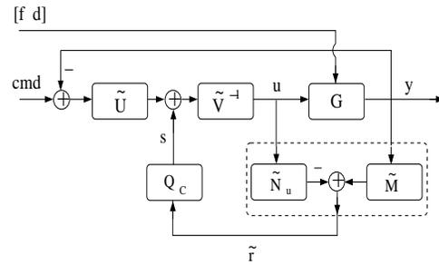
Fig. 2. Fault Tolerant GIMC-Youla Structure.
