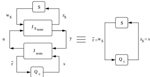
Fig. 8. Closed loop  $(G(S), K(Q_c)) \equiv (S, Q_c)$ .
