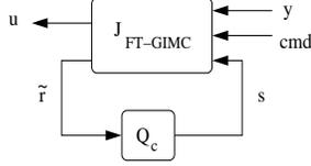
Fig. 3. Fault Tolerant - GIMC (lower LFT).
