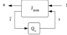
Fig. 1. Class of stabilizing controllers (lower LFT).
