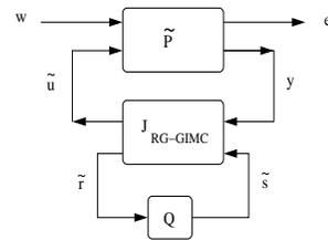
Fig. 5. Closed loop triad ( $\tilde{P}, J_{RG-GIMC}, Q$ ) [ $cmd = 0$ ].
