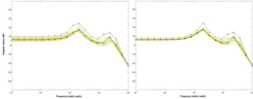
Fig. 4:  $LFT_A$  (left) and  $LFT_B$  (left) maximum singular value analysis: random (yellow), nominal (black \*) and worst-case gain (red +)
