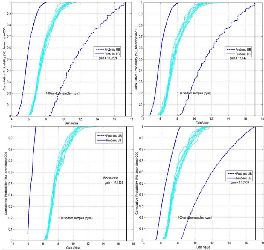
Fig. 8: Prob- $\mu$  bounds (blue) and MC (cyan) CDFs plus WCgain (vertical black): 20 freq-pts,  $LFT_A$  (top-row) vs  $LFT_B$  (bottom row) and Full  $\Delta$  (left column) vs No Bending  $\Delta$  (right column)
