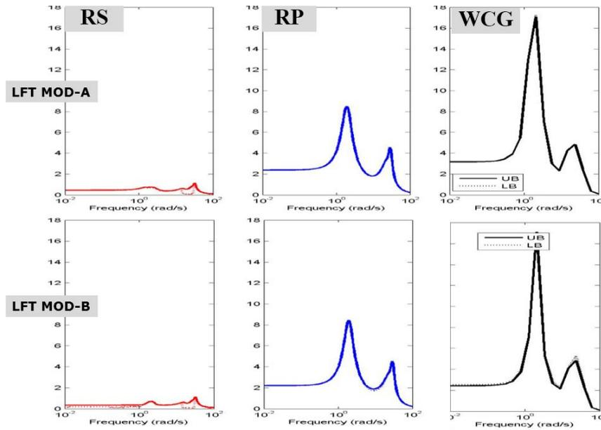
Fig. 7: WCG/RS- $\mu$ /RP- $\mu$  bounds for full uncertainty set:  $LFT_A$  (top) and  $LFT_B$  (bottom)
