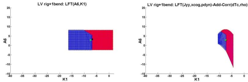
Fig. 3:  $LFT_A$  (left) and  $LFT_B$  (left) models eigenvalue analysis: stability (blue) and instability (red)
