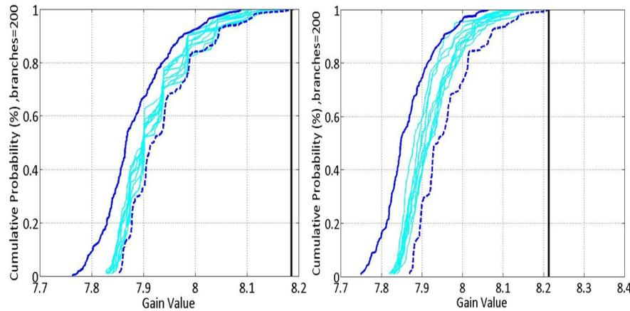
Fig. 9: Prob- $\mu$  bounds (blue) and MC (cyan) CDFs plus WCgain (vertical black) for  $LFT_A$  model: 200 freq-pts but only  $\Delta = (A_6, K_1)$  - pure real (left) and mixed real-complex (right)
