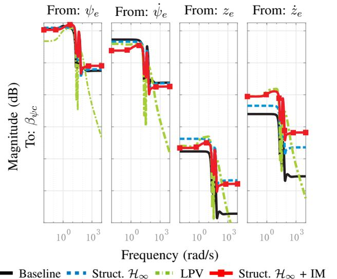
Fig. 8: Bode plot controller comparison at t=50s
