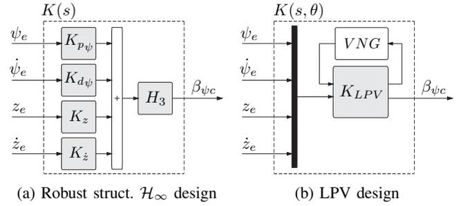
Fig. 4: TVC structure for the VEGA control designs
